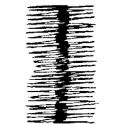
Top Too Loose or Bottom Too Tight
